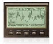
For signals that are readily demodulated, the OSCOR easily classifies threatening signals. Signals that are not readily demodulated are flagged for manual inspection.
