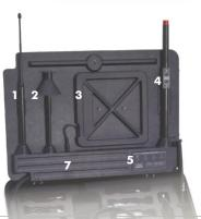
Patented fold-out antenna panel automatically selects the proper antenna. Pre-amp provides maximum sensitivity for the proper input. No unreliable cable connections or mismatched antenna inputs.
