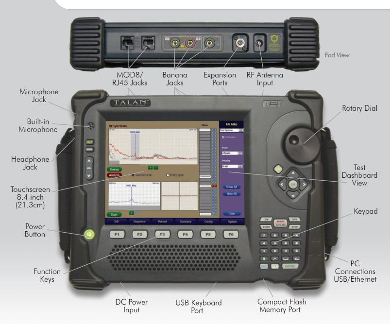
The TALAN provides a suite of tools in a single piece of equipment to accurately analyze phone lines for taps and other eavesdropping threats.
